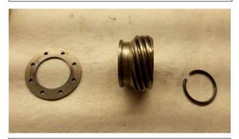
Thrust washer with holes in it slides 1<sup>st</sup> onto the spline shaft, then the speedometer drive gear, and then the keeper ring.
